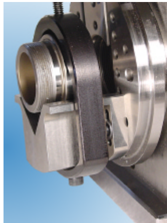
(Above) A standard 1/4 20 S.H.C.S. modified with a 45 degree angle on 2 sides and leaving a flat ground on the top, provides a 2 point clamp for very small parts. Having 2 pressure points rather than 1 minimizes distortion of the part.
