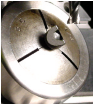
(Above) A standard 1/4 20 S.H.C.S. modified with a 45 degree angle on 2 sides and leaving a flat ground on the top, provides a 2 point clamp for very small parts. Having 2 pressure points rather than 1 minimizes distortion of the part.
