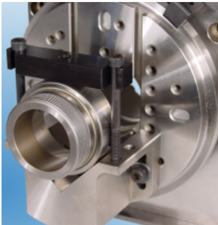
(Above) A standard 1/4 20 S.H.C.S. modified with a 45 degree angle on 2 sides and leaving a flat ground on the top, provides a 2 point clamp for very small parts. Having 2 pressure points rather than 1 minimizes distortion of the part.
